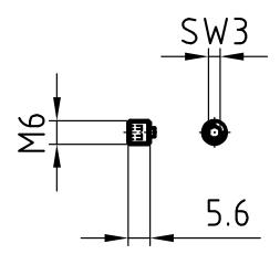
Standard version Screw with hexagon socket M6 x 8 mm Stainless steel, hardened
